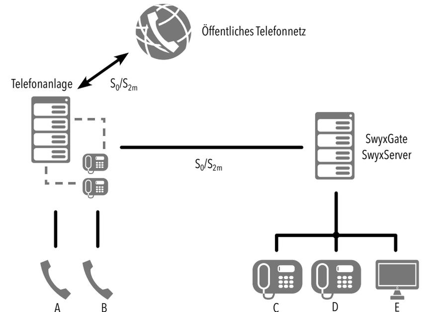
Abb. 3-3: SwyxGate an PBX angeschlossen
